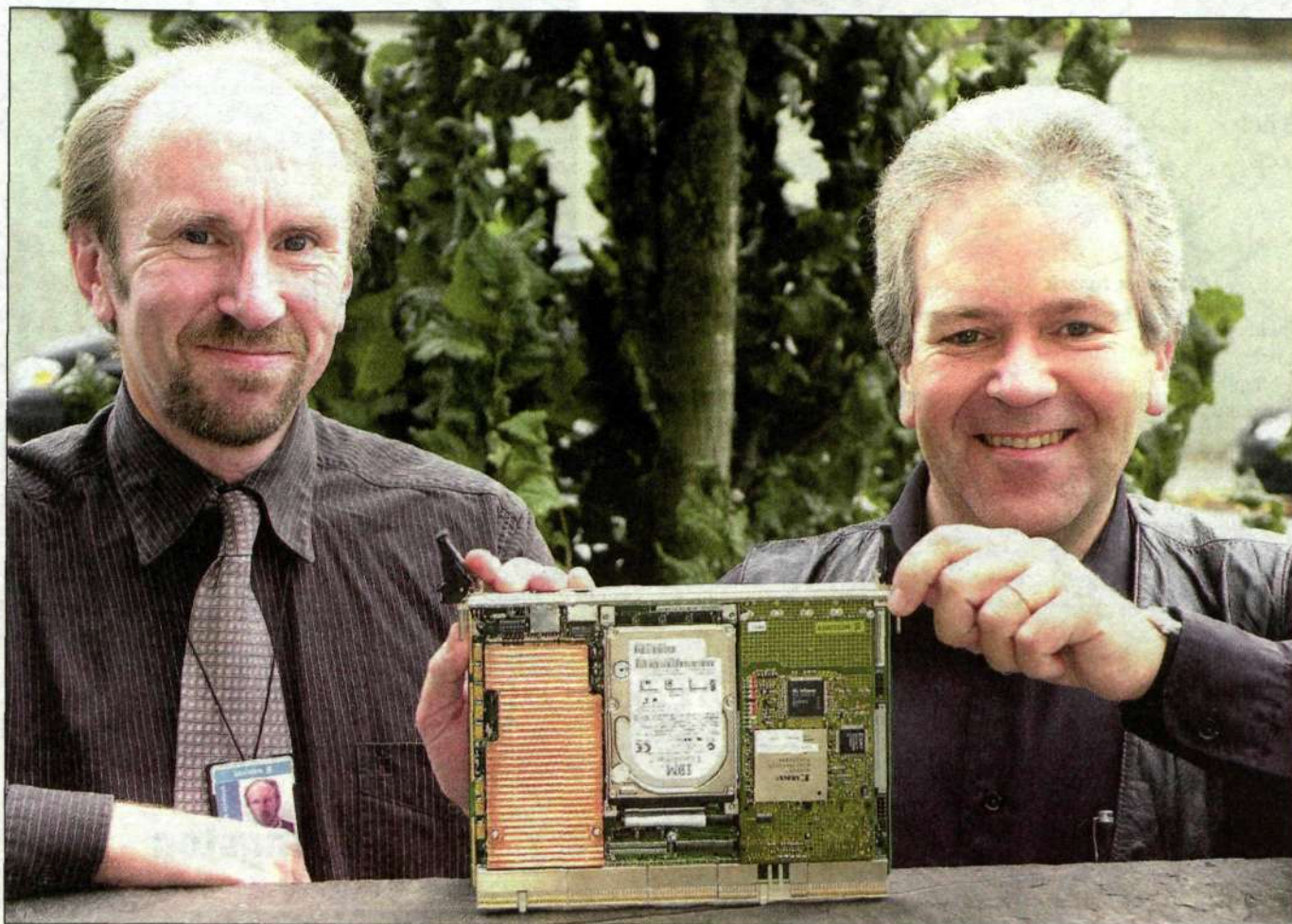
Olle Hergren and Jörgen Tränk show the new SS7 Stack-on-a-Card. The green card is the network card that was developed in-house. A hard disk is mounted at the center of the board, while an Intel Pentium III central processor is located to the left. Note also the large circuit in the middle of the communication card, which is an FPGA (Field Programmable Gate Array) circuit that allows software and upgrades to be downloaded dynamically without replacing the card.
