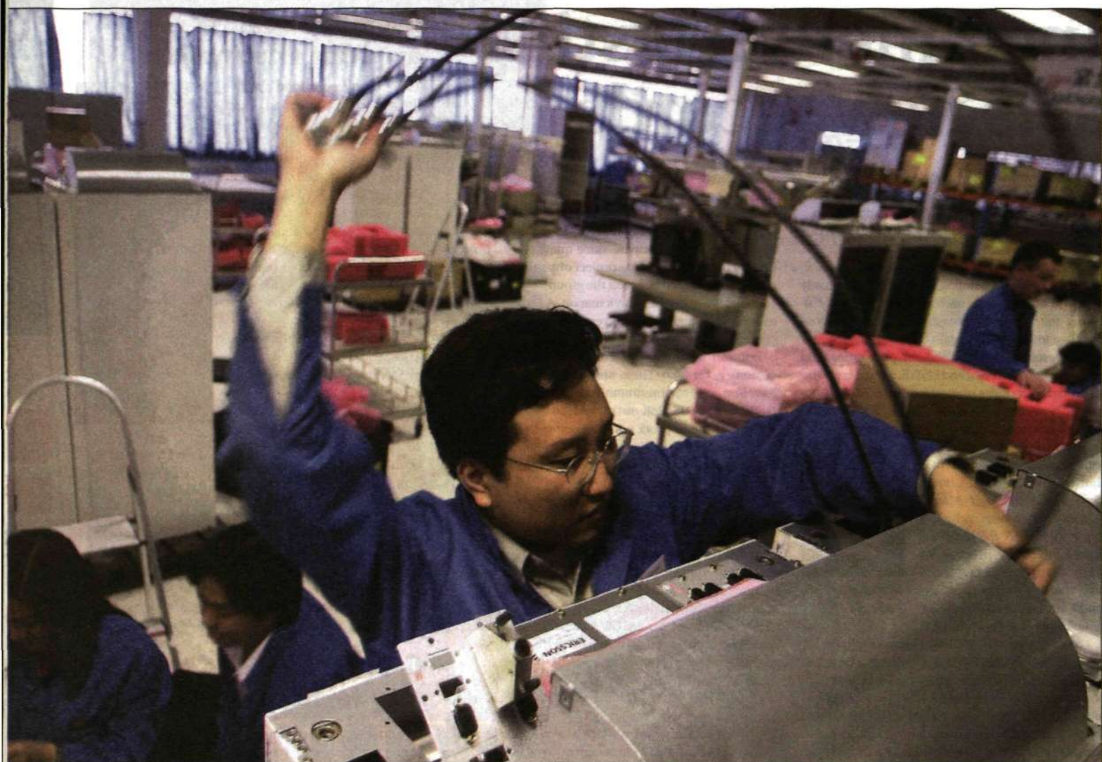
Since a new law was passed four years ago, nearly all systems equipment for the Chinese market has been produced within the borders of China. Ericsson's plants are now among the company's largest subsidiaries. The picture shows the final stages in the assembly of a radio base station at BMC in Beijing. PHOTO: LARS ASTRÖM
