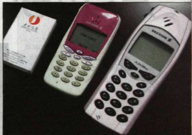
The A2638 was the first Ericsson phone with a built-in antenna. This model was adopted from the A2618 and developed in China to meet demand there. Other phones have followed, such as Ericsson's smallest phone, the T66, pictured on the left. Both models are manufactured at the Nanjing plant.
