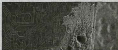
An image of a damaged circuit obtained with an electron microscope. A short circuit, caused by lightning or something else, has damaged the silicon and sent the component to the IC graveyard.
