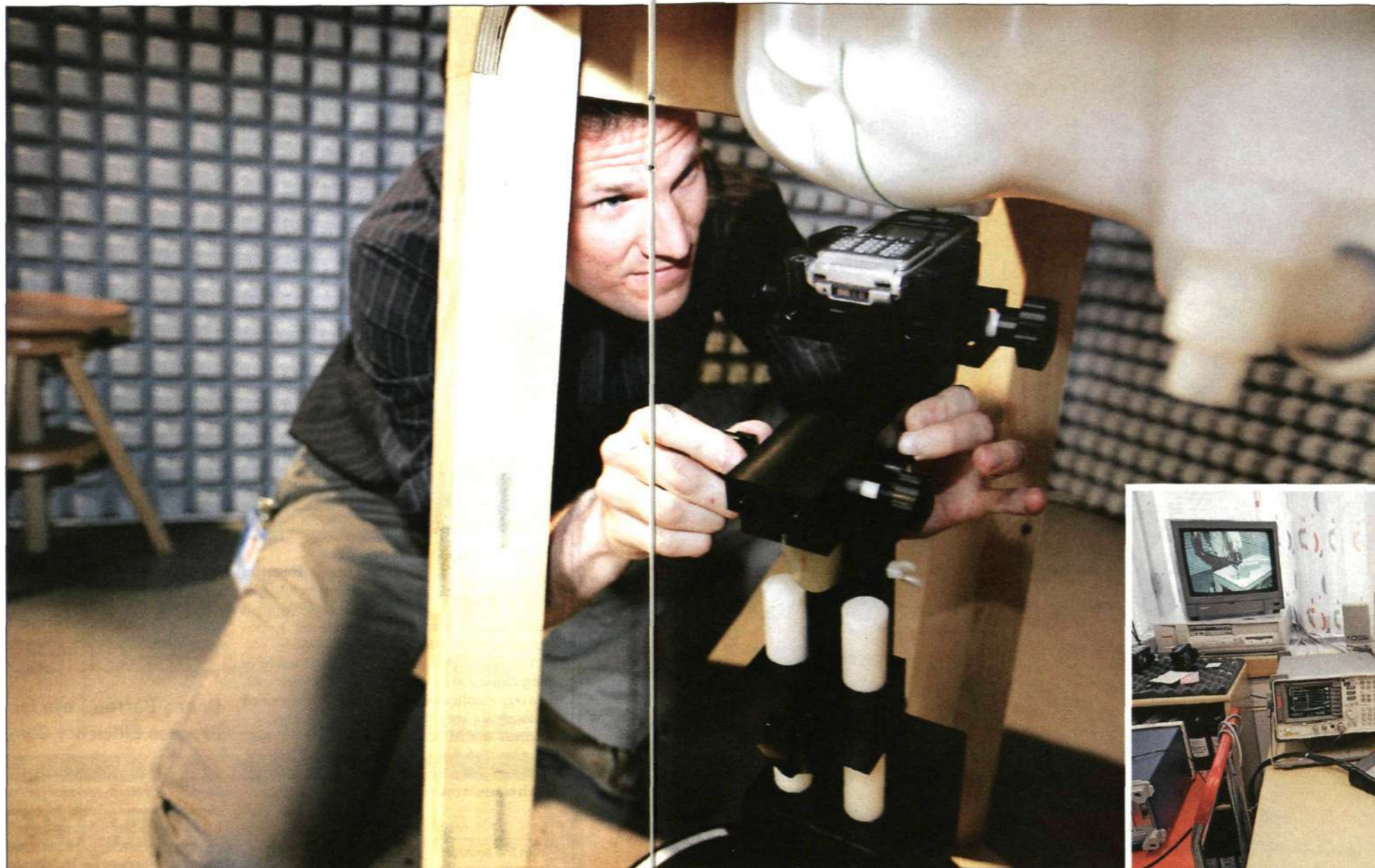
All Sony Ericsson telephone models undergo SAR tests before they are launched. The process uses a head-shaped model filled with liquid that has the same electrical properties as the human head. The measurements determine whether the telephones meet limits for exposure to radio waves.
