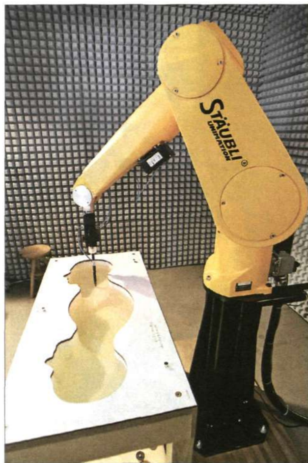
All Sony Ericsson telephone models undergo SAR tests before they are launched. The process uses a head-shaped model filled with liquid that has the same electrical properties as the human head. The measurements determine whether the telephones meet limits for exposure to radio waves.
