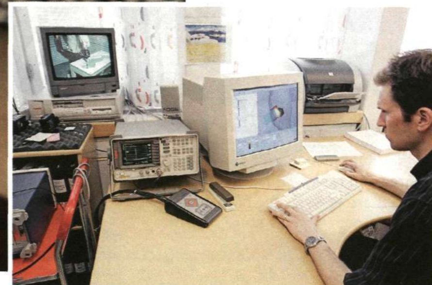
Lennart Hamberg attaches a telephone to a holder under one side of the heads. He specifies the measurement points from the computer.
