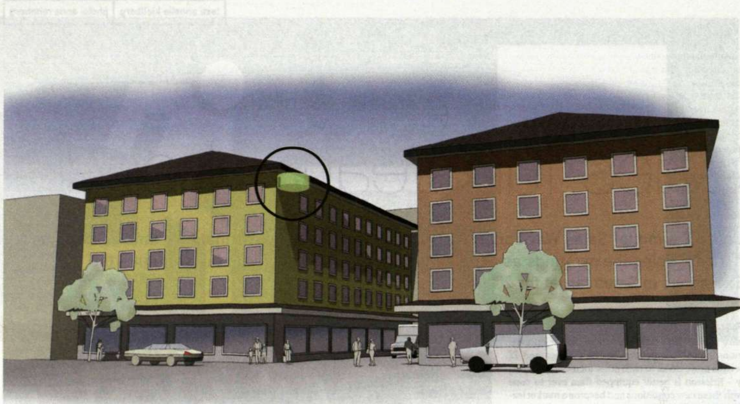
The green area shows the zone around the antenna where the field can be higher than the established exposure limit. On the street the field is below 1 percent of the limit.
