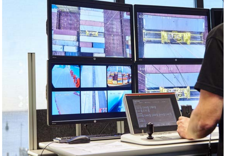
Figure 3: Remote operation system Photographer: Hans Nordlander
