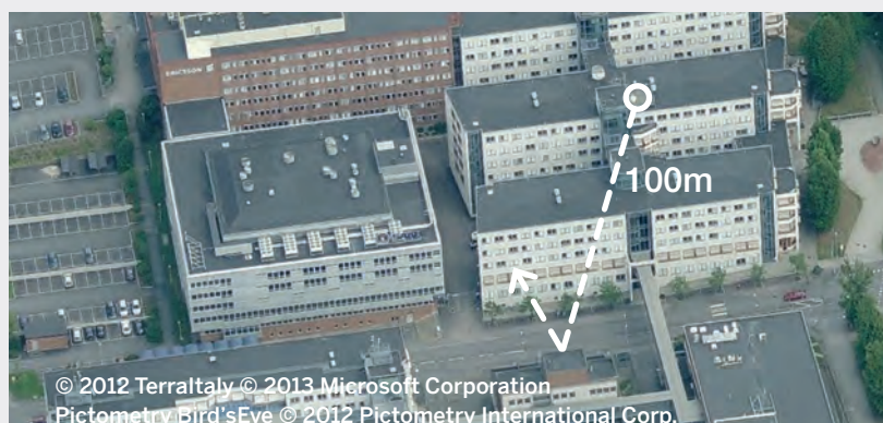
FIGURE 4A Test site for NLOS backhaul – reflection
