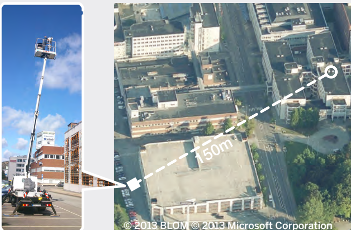
FIGURE 3A Test site for NLOS backhaul - diffraction
