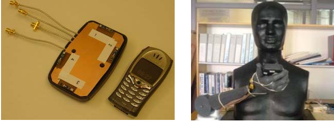
Fig. 1. The terminal with case open (compared to a common-size mobile phone) and the user phantom in the multimedia mode.
