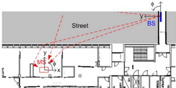
Fig. 2. Site map of measurements with the BS position and the MS (3D robot) position marked. A few example (typical) rays are drawn.
