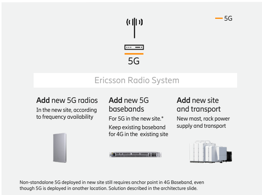
Figure 12: Case 2, NSA 5G deployment with 4G in low/mid bands and 5G in high bands.
