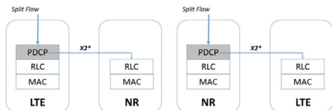
Fig. 1: A common PDCP layer aggregation for 5G AIs.
