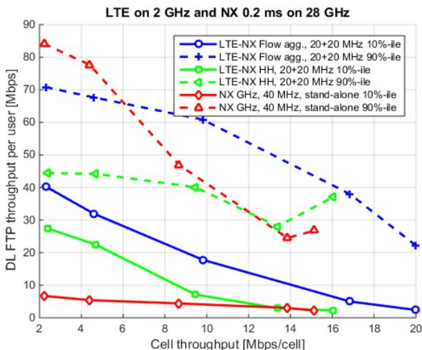
Fig. 6: User throughput vs. cell throughput (load) for NR (0,2 ms TTI, 28 GHz) and evolved LTE (1 ms TTI, 2 GHz) in fast user plane switch case.
