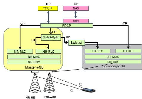
Fig. 2: Evolved LTE and NR protocol stack for fast switching.
