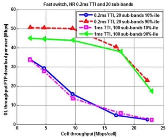
Fig. 5: User throughput vs. cell throughput (load) for NR (0.2 ms TTI, 2.6 GHz) and evolved LTE (1 ms TTI, 2 GHz).
