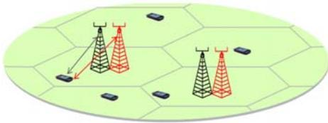
Fig. 3: 5G system topology: evolved LTE and NR co-sited deployment
