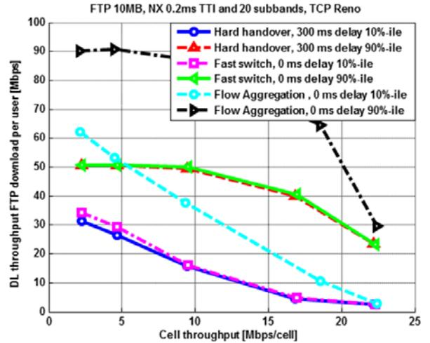
Fig. 4: User throughput vs. cell throughput (load) for NR (0.2 ms TTI) and evolved LTE (1 ms TTI).
