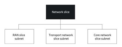
RAN slicing secures the allocation of limited radio resources to support SLA fulfillment for the associated UEs and services.
