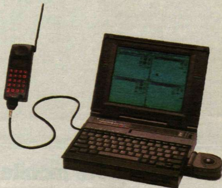
Texas TravelMate notebook computer with Ericsson modem connected to an Ericsson handheld mobile phone NH 97.
