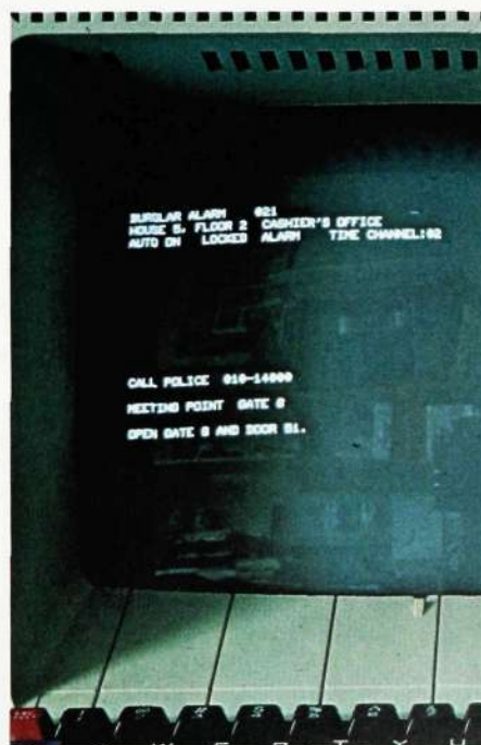
Fig. 4 Visual display screen and operator panel. The information on the screen consists of section number, object address, object state and proposed measures
