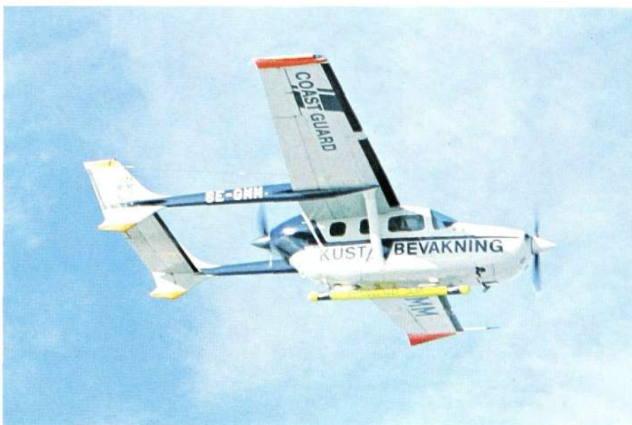
Fig. 1 The Coast Guard Cessna 337 with an SLAR antenna pod
