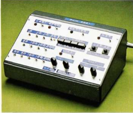
Fig. 6 Control box for remote control of the supply sources (network, motor generator, variac, battery, cell switches and rectifiers) and for the control of different loads
