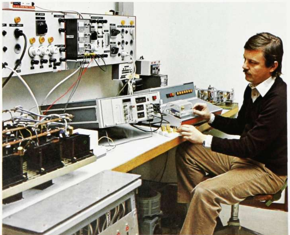
Fig. 7 A long-term test room. Power transistors are undergoing cyclic load testing. The instrument on the right is a switch time tester for fast power transistors, designed by LM Ericsson
