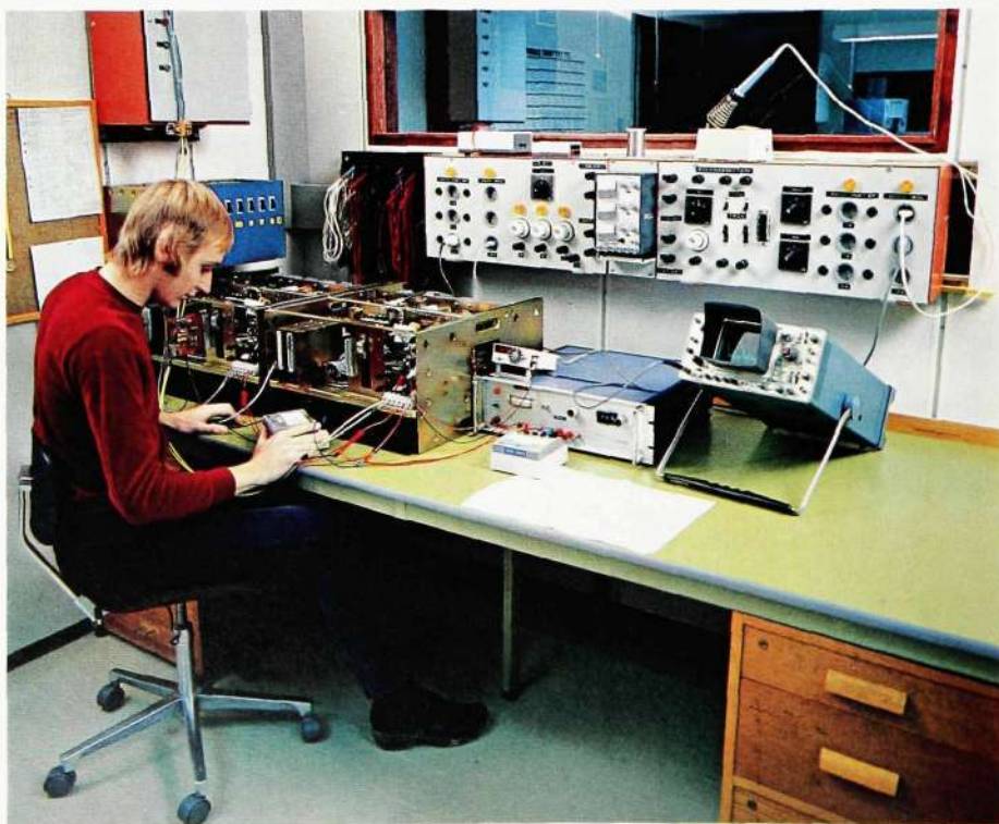
Fig. 1 The development of AC system BZV 102 was carried out in LM Ericsson's modern power supply laboratory in Stockholm. Two inverters that form part of the system are being tested here
