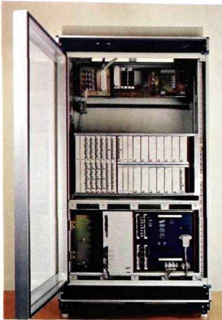
Fig. 9 Rectifier BMT 241 (4 A) in transmission equipment ZAE 12-1. The rectifier contains a separate distribution fuse. The rectifier can be supplemented by a standard printed board assembly for automatic charging and will then function as a battery charger
