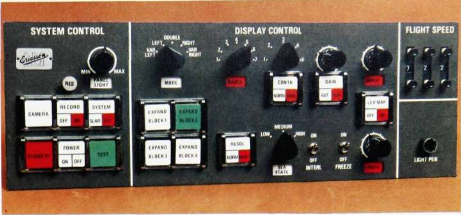
Fig. 7 Control panel. All system functions are controlled from the panel except the luminance and contrast of the TV monitor
