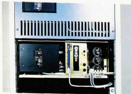
Fig. 6 Inverter BMS 301, with its front plate removed, seen from the front when mounted in the rack. The inverter is operated by two push buttons, start and stop, mounted on one printed board assembly to the left in the unit
