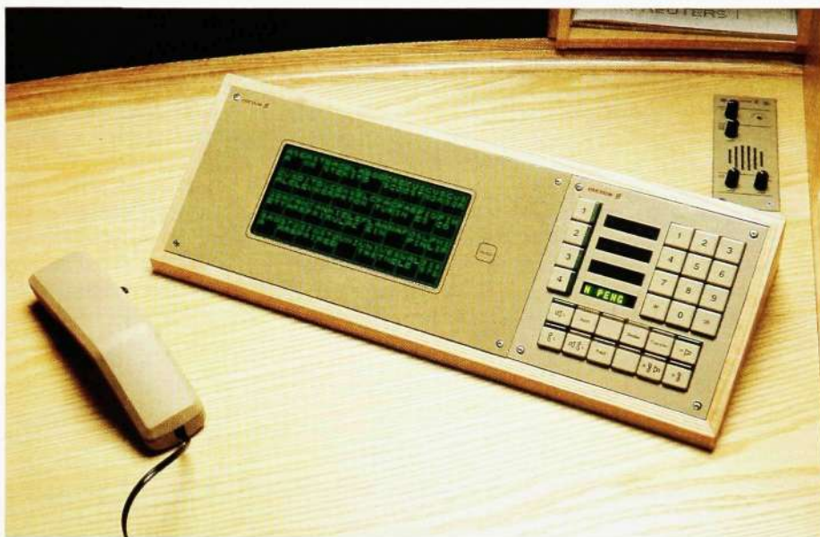
Fig. 3 The touch screen terminal contains a direct access panel, an indirect access panel, line buttons, function buttons, a push-button set and a control unit. Two handsets, two loudspeakers and a microphone can be connected to the terminal
