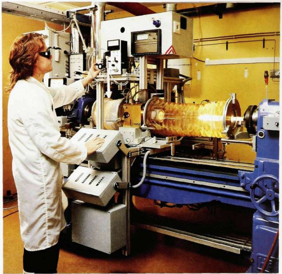
Fig 6 A preform being jacketted in an IMCVD lathe. The brass microwave cavity unit can be seen just to the right above the upper control panel. The heated quartz tube, which is strongly luminescent, is surrounded by flexible metallic screens which prevent leakage from the cavity
