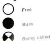
Fig. 4 The button panel of DIALOG 2752, with the names of the team members marked above the programmable buttons. Each button has an LED that shows whether the extension is free, busy or being called
