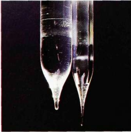
Fig 7 Preforms from the two processes, MCVD on the right and IMCVD on the left. An MCVD preform of 50 cm gives approximately 15 km of fibre and an IMCVD preform of the same length approximately 50 km
