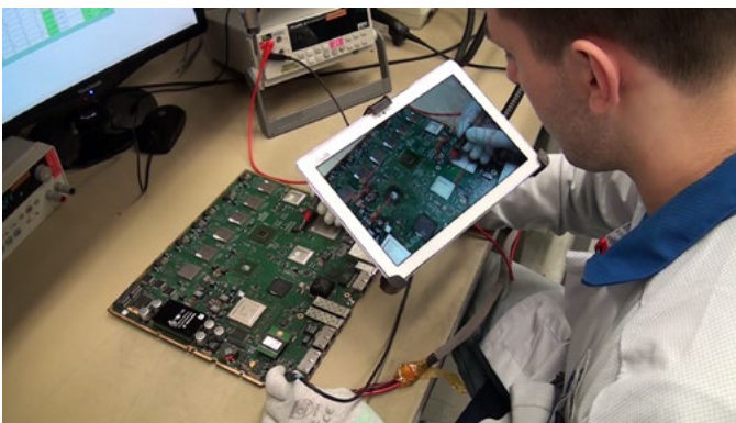
Now, instructions are shown as an overlay on a tablet screen or AR headset
