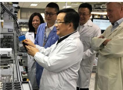
Now, more than 50 % of the high-precision screwdrivers have been fitted with real-time motion sensors attached to NB-IoT modules. Every eight hours, the module transmit about 100 bytes of data indicating the utilization time.
