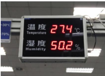
Environmental conditions, such as humidity, dust levels, and air temperature, need to be maintained within specific parameters to ensure product quality while storing. Although wired sensors can monitor the climatic conditions, NB-IoT has made it cost-effective to use wireless sensors, which can be deployed quickly and then moved from place to place, as required.
