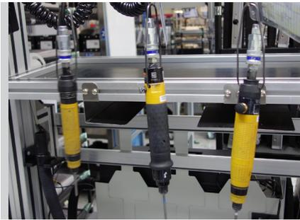
Before implementing NB-IoT, maintenance of the factory's more than 1,000 high-precision screwdrivers relied on hand-written records. The screwdrivers (which cost US\$1,500 each) require routine calibration and lubrication based on utilization times, to secure the quality and performance of the radio products.
