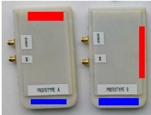
Fig. 1. Illustration of antenna location in dual-antenna devices (A and B) in a medium-size smartphone form factor.
