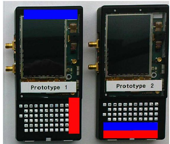
Fig. 2. Illustration of antenna location in dual-antenna devices (1 and 2) with dimensions of a larger smartphone.
