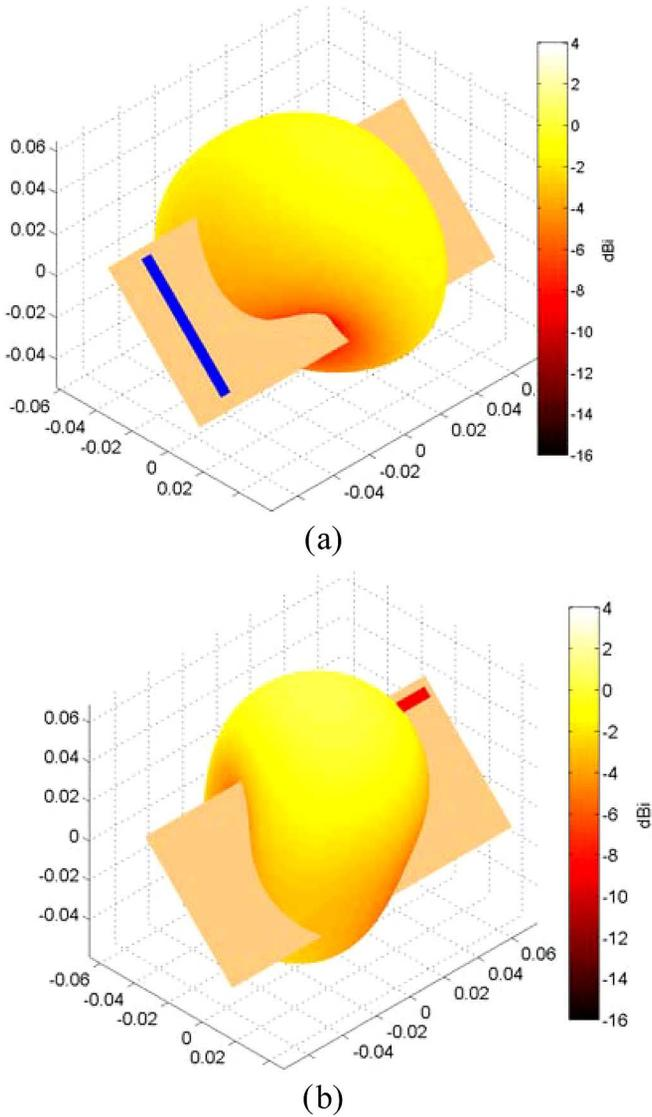
Fig. 3. Measured embedded total power radiation patterns of device 1 tilted 45° backwards at 750 MHz. (a) Main antenna. (b) Diversity antenna.
