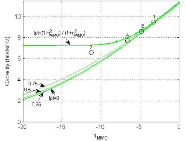
Fig. 4. Channel capacity at 20-dB SNR as a function of MIMO efficiency assuming a spherical uniform power spectrum of the incident field and with the magnitude of the complex correlation as a parameter.
