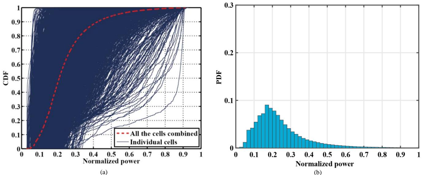
Fig. 2. (a) Empirical cumulative distribution function (CDF) of normalized 3G RBS output power for all 2,475 cells during the week-long measurement. (b) Probability Density Function (PDF) of the red curve in Fig. 2a.
