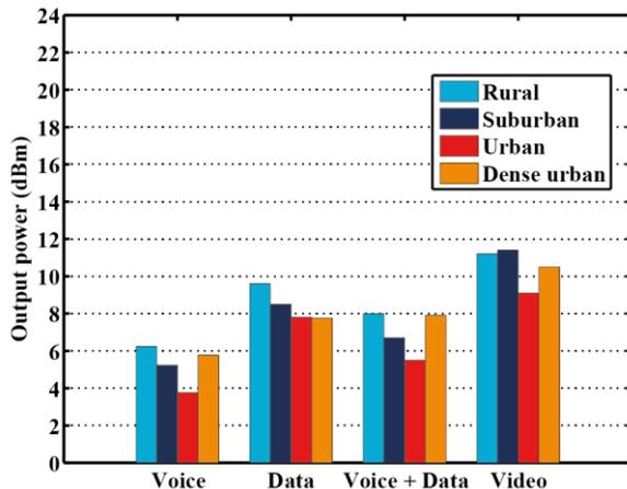
Fig. 6. Mean 3G user device output power for different applications in different environments.
