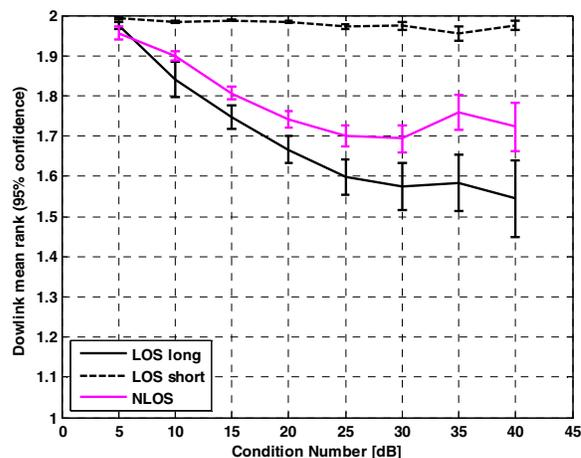
Fig 10. Condition Number vs mean transmission rank.
