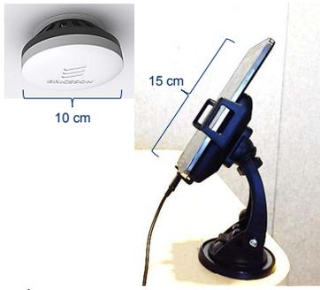
Fig. 1. Test equipment.
