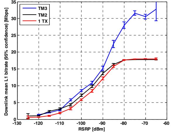
Fig 4. RSRP vs throughput for different MIMO configurations NLOS
