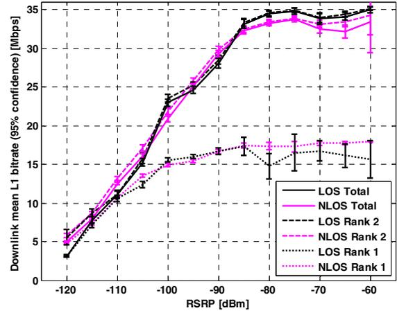
Fig 7. RSRP vs throughput with TM 3 for the long walk routes.
