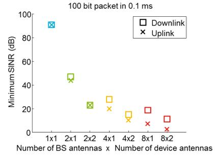
Fig. 2. Minimum required SINR to achieve the reliability and latency requirements for different antenna configurations assuming maximum ratio combining and QPSK modulation with a  $\frac{1}{2}$ -rate convolutional code.
