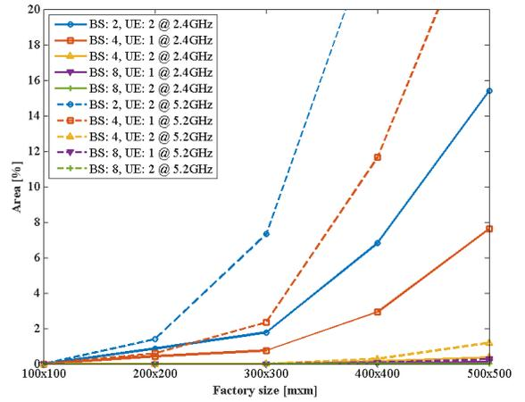
Fig. 3.b. Uplink out-of-coverage area assuming a single-cell deployment.
