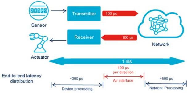
Fig. 1. Distribution of the end-to-end latency assuming a 100- $\mu$ s air interface delay [7].
