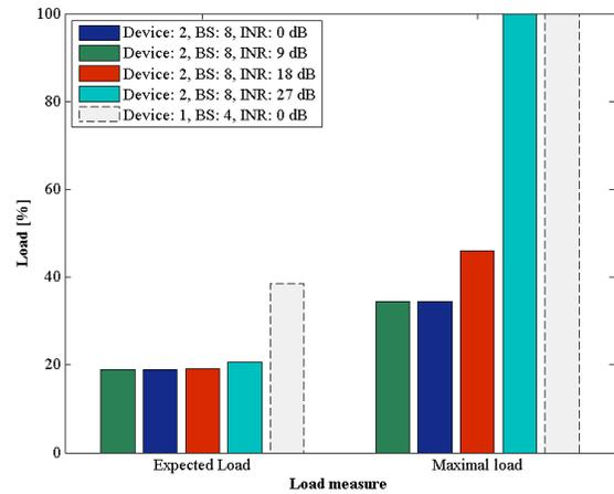
Fig. 7.b. Uplink system capacity when interference-present environment is assumed for a 100 m x 100 m factory floor.
