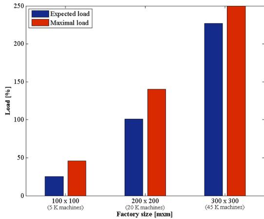
Fig. 6.a. Downlink system capacity when interference-mitigated environment is assumed for different factory floor layouts.
