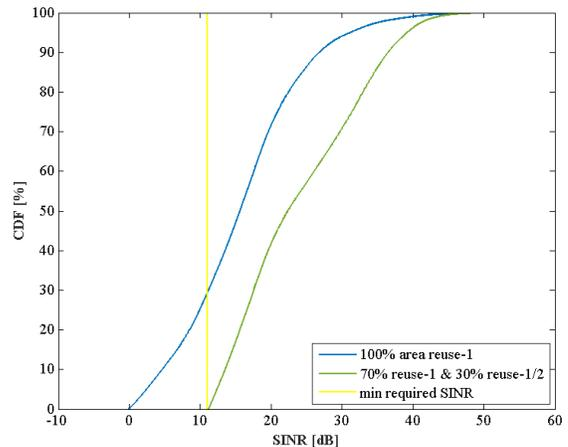
Fig. 5.a. Downlink SINR CDF of frequency partitioning where 70% of the area operates on reuse-1 and 30% on reuse-1/2.
