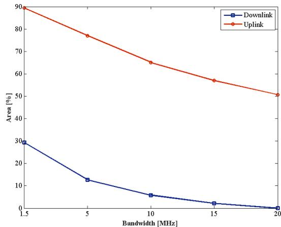
Fig. 4. Out-of-coverage area assuming a 2-cell deployment with frequency reuse-1 at 5.2 GHz.
