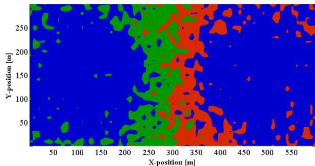
Fig. 5.b. Illustration of downlink frequency partitioning assuming a 2-cell deployment where 70% of the area operates on reuse-1 (blue region) and 30% on reuse-1/2 (green and red regions).
