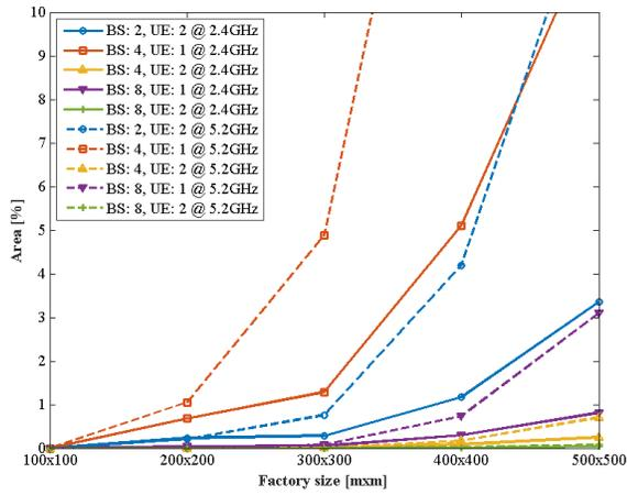
Fig. 3.a. Downlink out-of-coverage area assuming a single-cell deployment.
