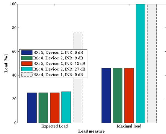
Fig. 7.a. Downlink system capacity when interference-present environment is assumed for a 100 m x 100 m factory floor.
