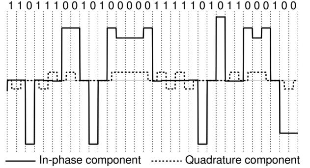
Fig. 4: CAPS-3 signal for  $\alpha = 0.1$  and  $\beta = 0.4$ . Here the intensity of the signal components is represented, but with the sign of the corresponding electrical field.
