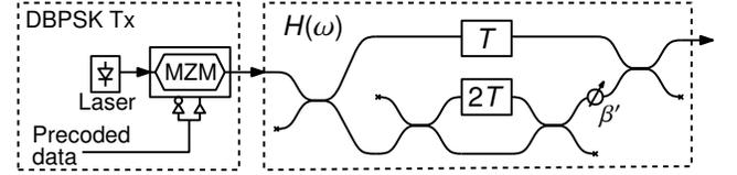
Fig. 10: IQ-DBPSK transmitter.
