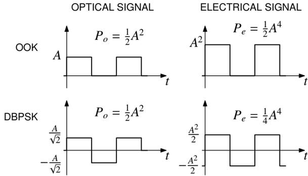
Fig. 1: OOK and DBPSK (lowpass equivalent) optical and electrical signals. The DBPSK electrical signal is polar because it is demodulated by an optical differential interferometer and detected by a balanced receiver.
