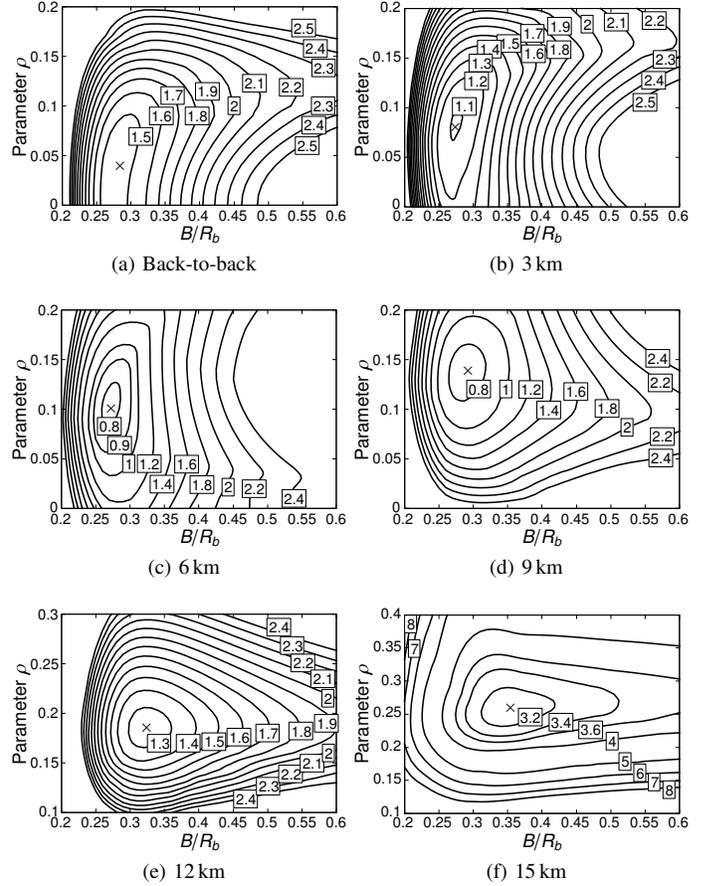
Fig. 13: IQ-duobinary contour plots of  $E_b/N_0$  penalty at  $\text{BER} = 10^{-3}$  vs  $\rho = g_2/g_1$  and the bandwidth  $B$  of the electrical filter at the transmitter (same fiber lengths and reference as in Fig. 12).
