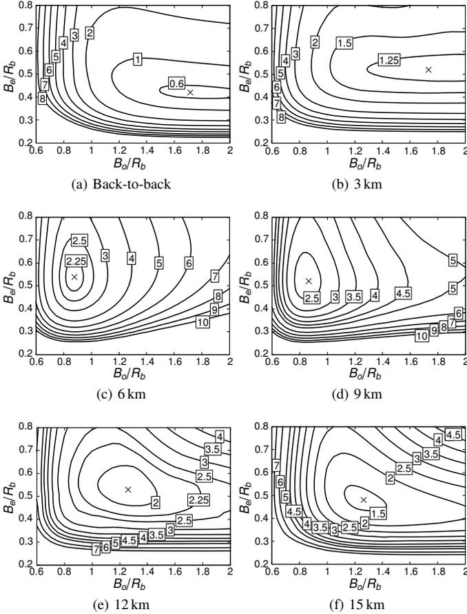
Fig. 12: CAPS-3 contour plots of  $E_b/N_0$  penalty at  $\text{BER} = 10^{-3}$  vs electrical ( $B_e$ ) and optical ( $B_o$ ) filter bandwidths for six fiber lengths (reference is the performance of an OOK system in back-to-back configuration).
