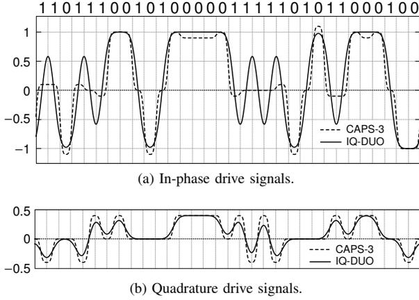
Fig. 8: Nested MZM electrical drive signals for CAPS-3 ( $\alpha = 0.1$  and  $\beta = 0.4$ ) and IQ-duobinary ( $g_2 = 0.2g_1$ ) for the given binary sequence. The IQ-duobinary electrical filter is Gaussian shaped with bandwidth  $R_b/3$ , while a bandwidth of  $0.8R_b$  was assumed for CAPS-3. The amplitudes are relative to the bias voltage and are normalized to the MZM  $V_\pi$ .
