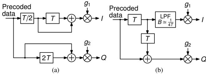
Fig. 6: Block diagrams for the generation of in-phase (I) and quadrature (Q) components. The duobinary in-phase component is ideal in (a) and obtained by filtering in (b).
