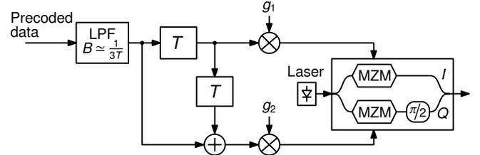
Fig. 7: IQ-duobinary transmitter.
