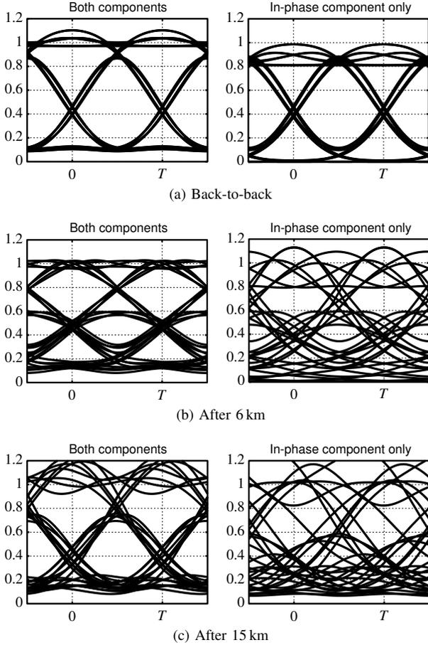
Fig. 5: Eye diagrams of the CAPS-3 signal in Fig. 4 after filtering and photodetection. Only the in-phase component was transmitted for the diagrams on the right side.
