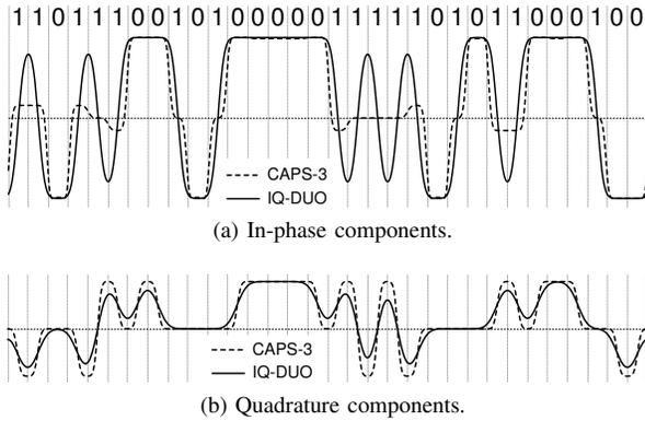
Fig. 9: Electrical fields at the output of the nested MZM corresponding to the drive signals in Fig. 8. The MZM is taken to have infinite extinction ratio.
