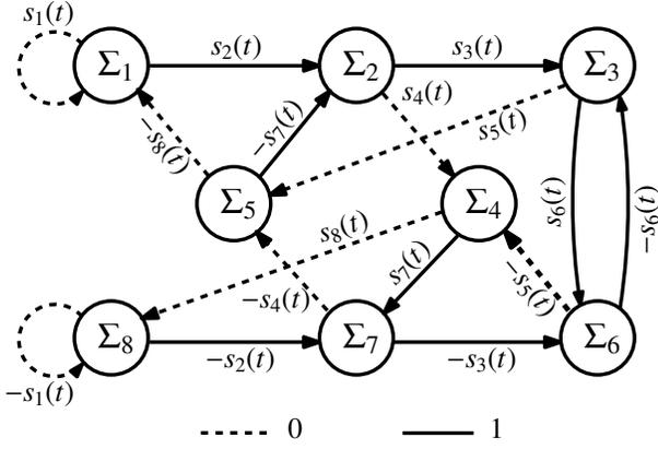
Fig. 2: State diagram of a CAPS-3 code.
