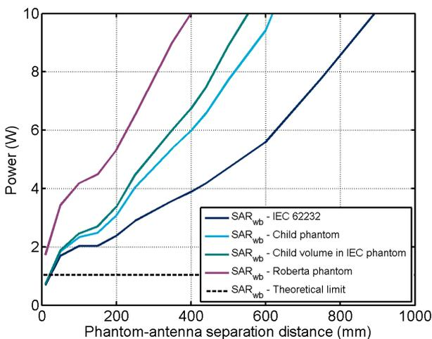
Figure 4. Comparison between different approaches for measuring child whole-body SAR ( $f = 2100$  MHz).
