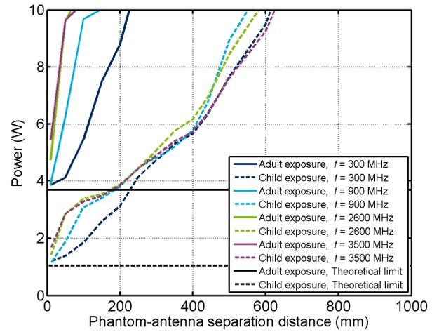
Figure 7. Comparison between general public whole-body SAR measurements results for adult and child exposure.
