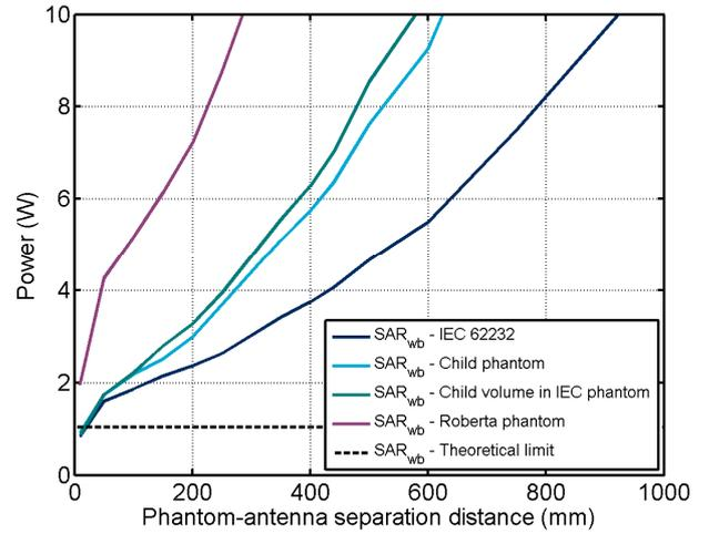
Figure 5. Comparison between different approaches for measuring child whole-body SAR ( $f = 3500$  MHz).
