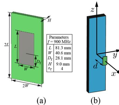
Figure 1. (a) Patch antenna element used for the analysis. (b) Adult (IEC) box-shaped phantom with patch antenna.
