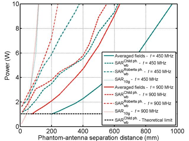
Figure 8. Comparison between SAR and field based general public exposure assessment methods ( $f = 450$  MHz &  $f = 900$  MHz).
