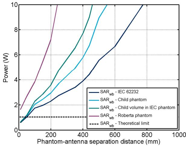
Figure 3. Comparison between different approaches for measuring child whole-body SAR ( $f = 900$  MHz).
