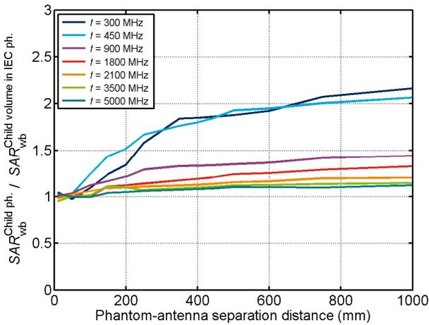
Figure 6. Bias introduced by assessing child whole-body SAR from the absorbed power within ‘child volume’ of the adult phantom for the patch antenna excitation.
