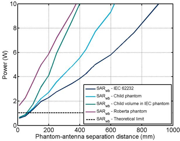
Figure 2. Comparison between different approaches for measuring child whole-body SAR ( $f = 450$  MHz).
