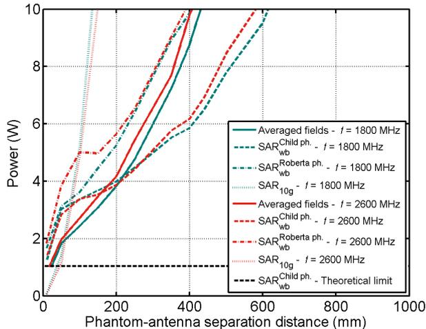
Figure 9. Comparison between SAR and field-based general public exposure assessment methods ( $f = 1800$  MHz &  $f = 2600$  MHz).
