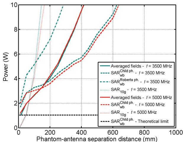
Figure 10. Comparison between SAR and field-based general public exposure assessment methods ( $f = 3500$  MHz &  $f = 5000$  MHz).
