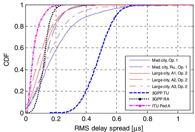
Figure 2. Cumulative distribution functions for the instantaneous rms delay spread measured in 3G networks in two different cities and two different operator networks. "A1", "A2" and "A3" denote data from different areas in the large city. "Ru" denotes data from rural areas in the vicinity of the mid-sized city. Simulated instantaneous rms delay spread distributions for three common channel models are plotted for comparison.
