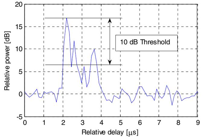
Figure 1. An example of a measured instantaneous power delay profile. This particular power delay profile has an rms delay spread of  $0.54 \mu\text{s}$  when considering only those peaks that are within 10 dB of the strongest peak.
