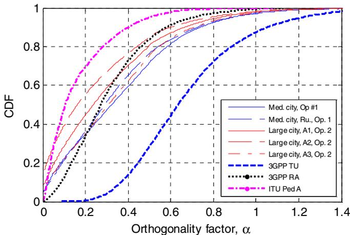
Figure 3. Cumulative distribution functions for the orthogonality factors measured in 3G networks in two different cities and two different operator networks. “A1”, “A2” and “A3” denote data from different areas in the large city. “Ru” denotes data from rural areas in the vicinity of the mid-sized city. Simulated instantaneous orthogonality factors for three common channel models are plotted for comparison.
