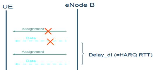
Figure 3. Error upon transmission of DL assignment.
