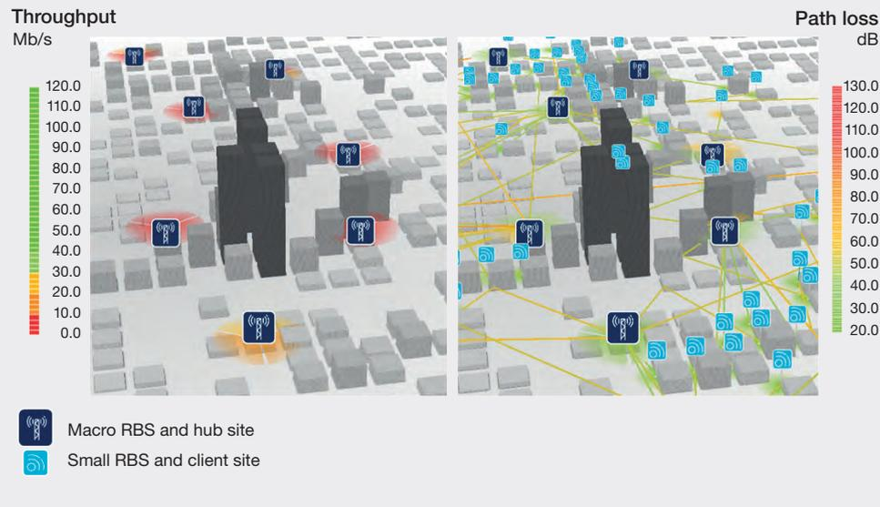
PtMP concept (described in this article). **Figure 2** illustrates the simulation scenario, showing two hubs providing wireless backhaul to two clients in an urban environment.
