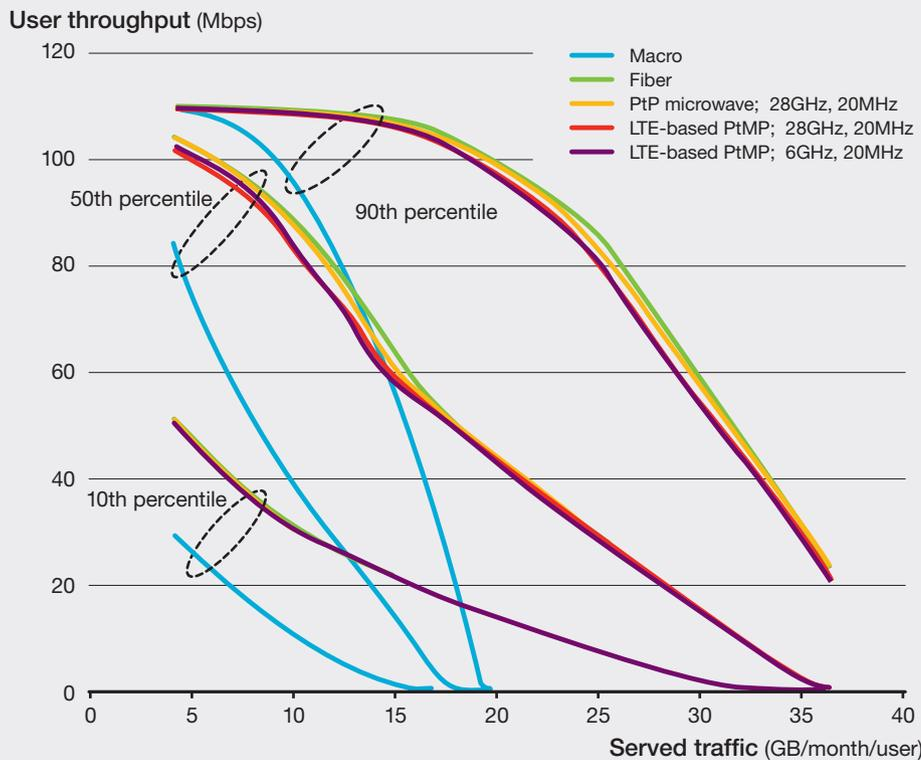
effect of access and backhaul, it has been shown that NLOS microwave backhaul in licensed spectrum up to 30GHz is a viable solution for dense small cell deployments in urban environments.
