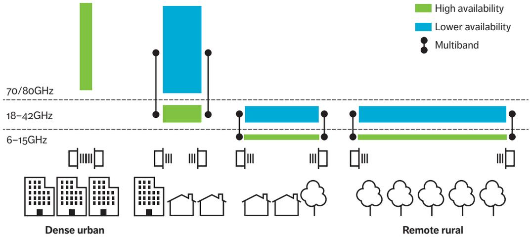
Figure 5: Efficient use of microwave backhaul spectrum
