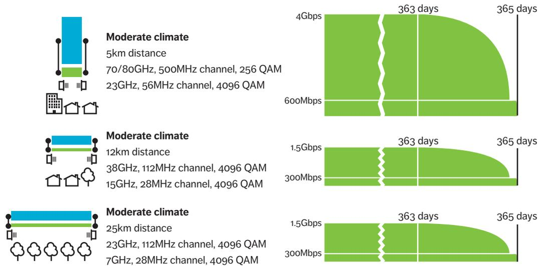
Figure 4: Examples of multiband microwave backhaul configurations
