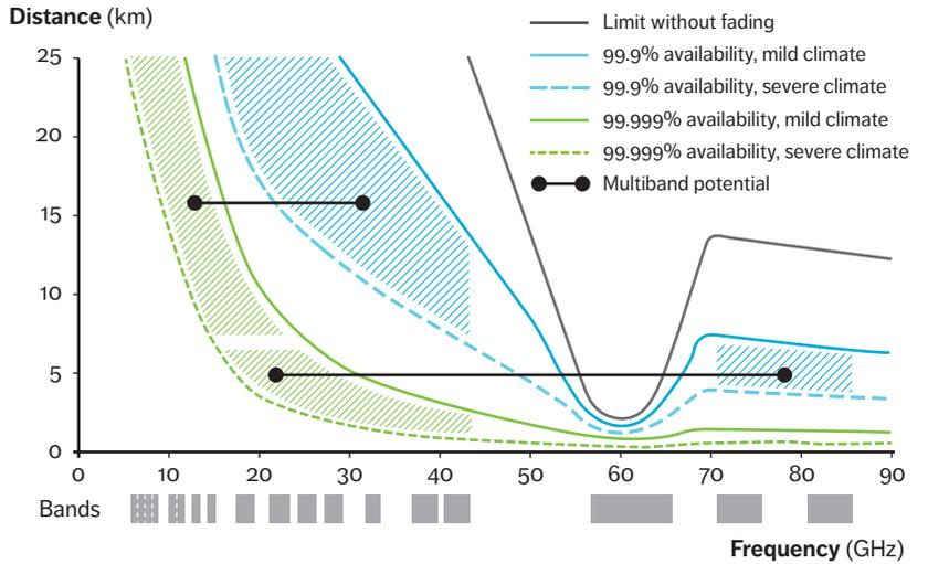
Figure 3: Achievable distances with high-capacity microwave backhaul
