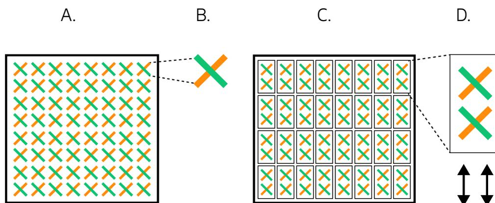
**Figure 2:** A typical antenna array (A) is made up of rows and columns of individual dual-polarized antenna elements (B). Antenna arrays can be divided into sub-arrays (C), with each sub-array (D) connected to two radio chains, normally one per polarization.
