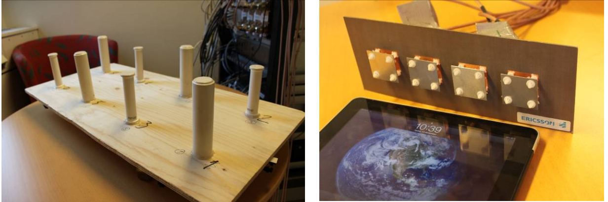
Figure 1 Reference UE antenna array (left) and compact array (right).
