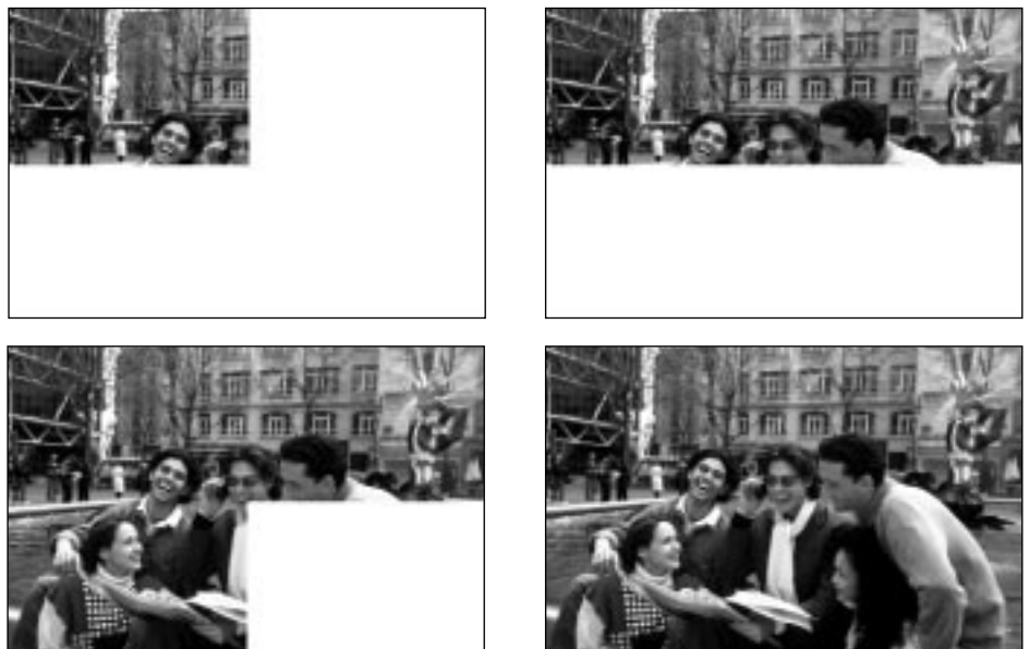
Figure 9 Progressive by position. The image is encoded in scan-line order so that the recipient first gets the top-left region of the image at full quality and resolution; the recipient then receives the remaining parts of the image from left to right and from top to bottom.
