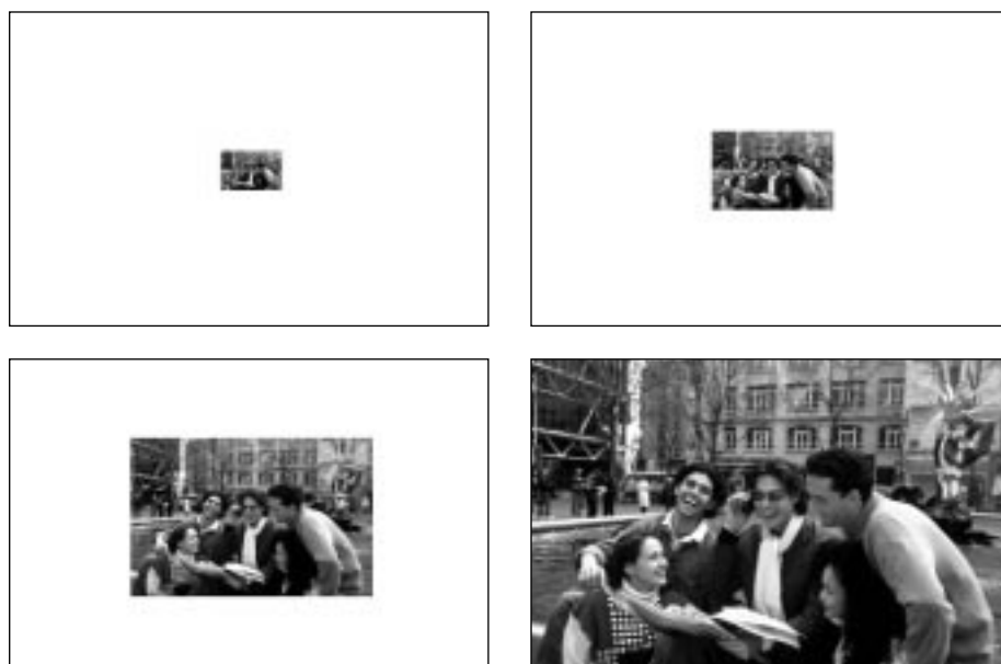
Figure 7 Progressive by resolution. The image is encoded so that the recipient first receives a low-resolution version of the image followed by the information needed to increase the resolution.
