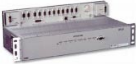
Figure 12 Photograph of a GPS system clock (GSC).
