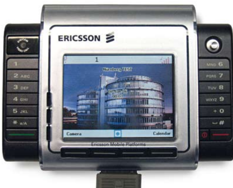
Figure 1 Accurate prototype form factor for demonstrating MBMS, VoIP and HSPA.
